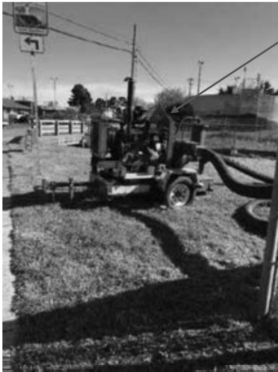
Stand-by portable pump for IPS. Pump 2 removed for repairs.
