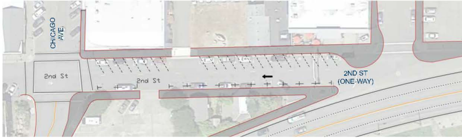
OPTION 1: PROVIDE ANGLED PARKING ALONG THE NORTH SIDE OF 2ND, ONE 11-FOOT TRAVEL LANE, AND PARALLEL PARKING ON THE SOUTH SIDE.
