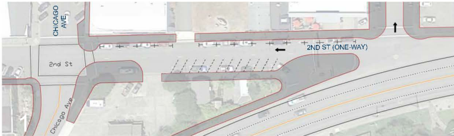
OPTION 2: PROVIDE ANGLED PARKING ON THE SOUTH SIDE, ONE 11-FOOT TRAVEL LANE, AND PARALLEL PARKING ON THE NORTH SIDE.
