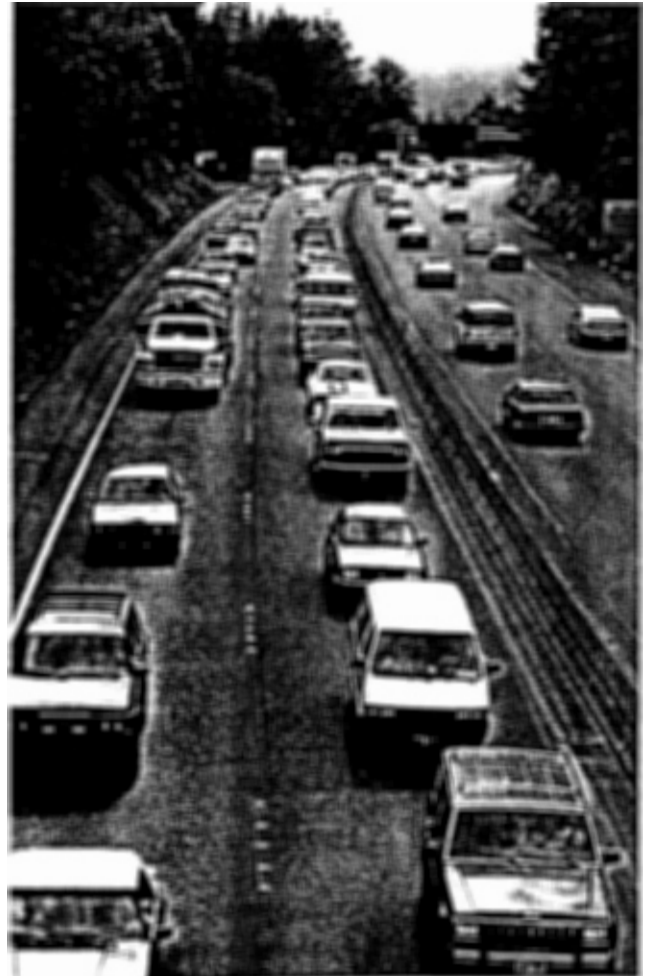
Traffic is bunching up and slowing down in all lanes of this freeway because traffic demand exceeds capacity.
