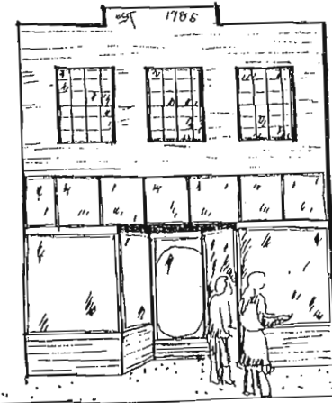
RECESSED ENTRANCE & STORE FRONT DISPLAY WINDOWS
